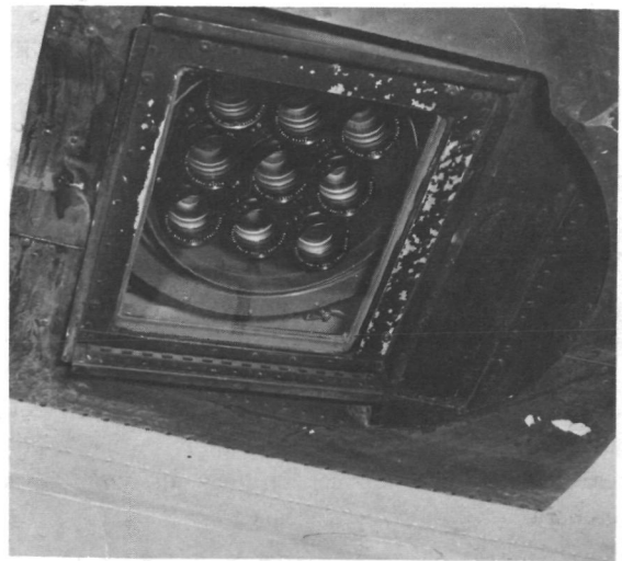
FIGURE 8. Itek nine-lens experimental multispectral camera.
