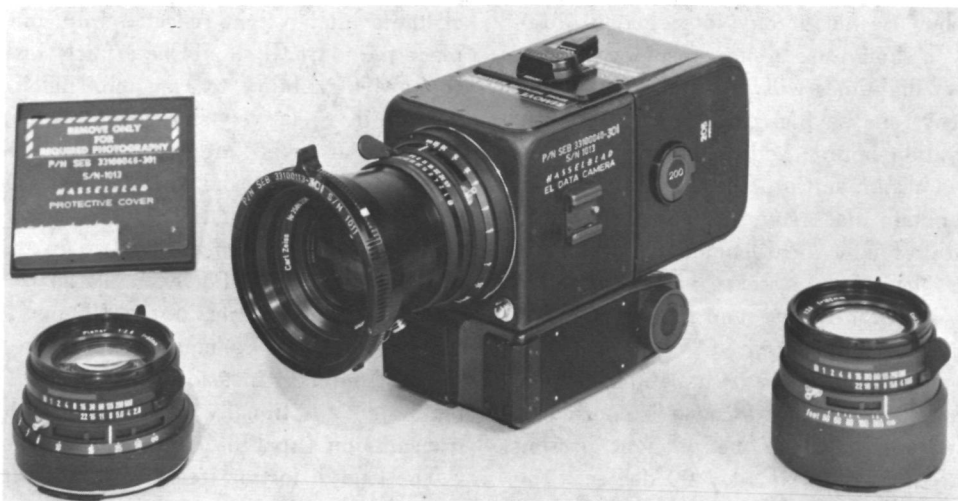
FIGURE 4. Hasselblad EL 70-mm data camera with reseau plate and interchangeable lenses (NASA photo).
