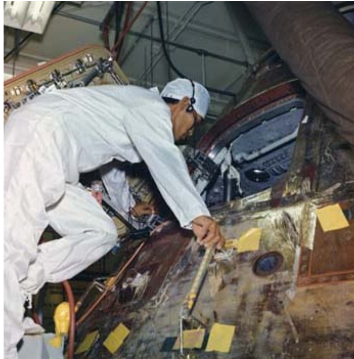
S69-45486.jpg - Landing and Recovery Division Systems Engineer John K. Hirasaki removing equipment and decontaminating of the interior of the Apollo 11 spacecraft inside the Lunar Receiving Lab.
