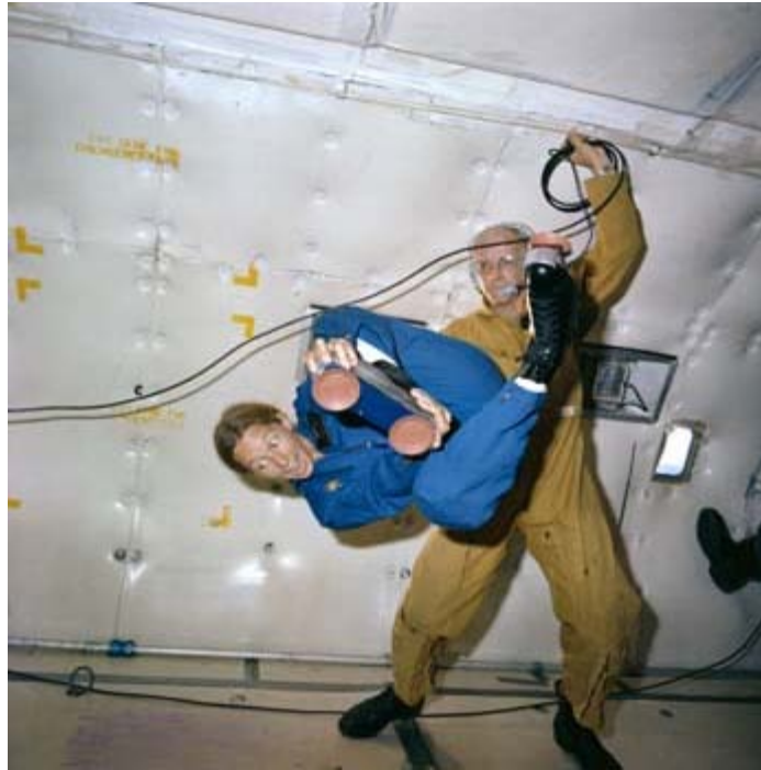
S79-35212.jpg - Astronaut Marsha Ivins on the KC-135 performing a Zero G evaluation of intravehicular activity (IVA) boots.
