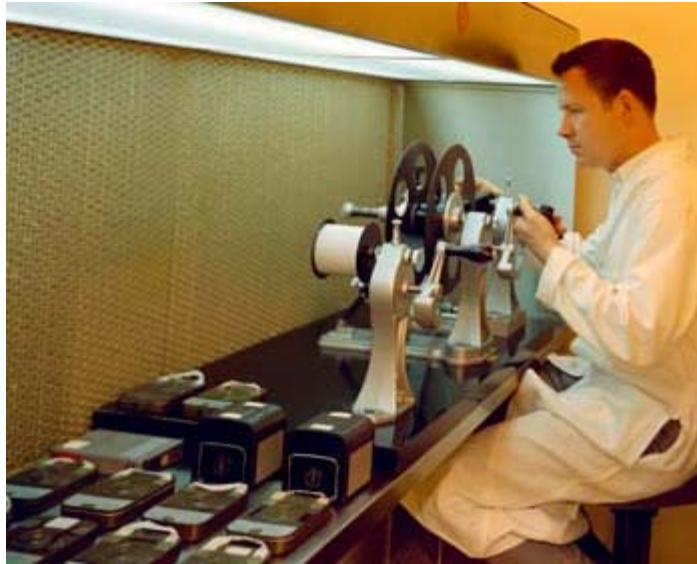
S69-25155.jpg - Part of the interleaving device that we used to interleave 16-millimeter and 70-millimeter film taken during the Apollo 11 mission. The film was put into light-baffled canisters and then into the autoclave for decontamination.
