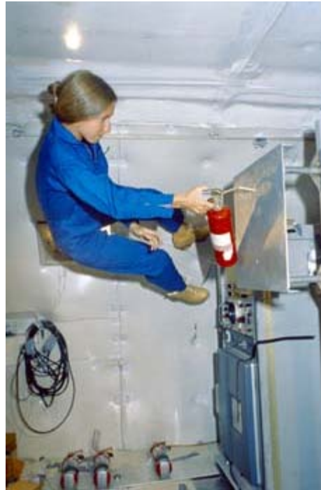
S78-31716.jpg - Astronaut Marsha Ivins on the KC-135 performing a Zero G evaluation of orbiter fire extinguishers.
