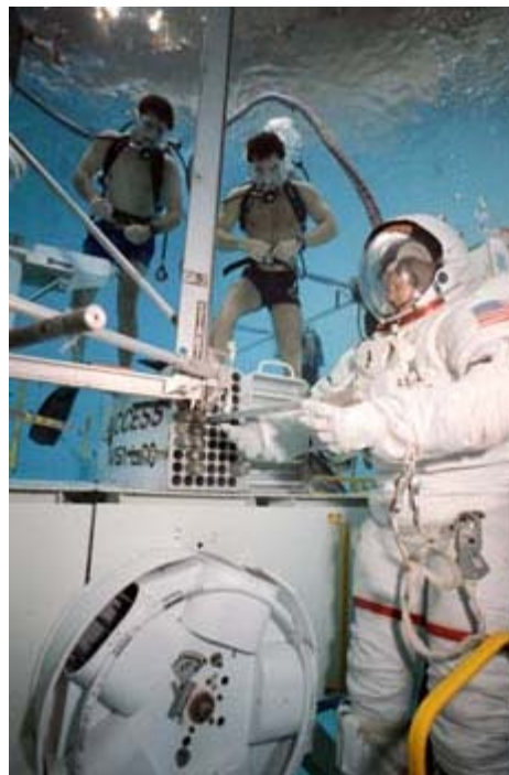
S89-38053.jpg - Underwater documentation using the AX-5 and MK III 8.3 PSI suits and the Space Shuttle 4 PSI suit in WETF evaluation runs, May 1989.
