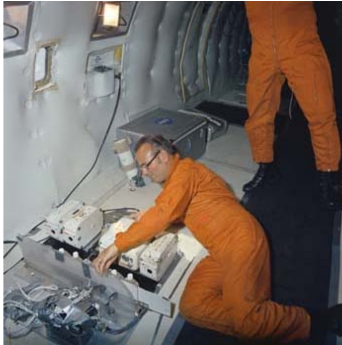
S75-29753.jpg - MIT zero gravity experiments onboard the KC-135. Six high-speed cameras were used to record the events.
