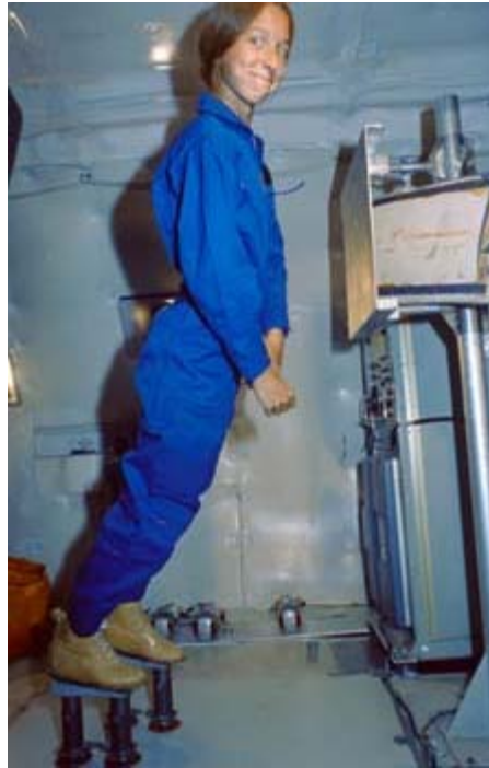
S78-31715.jpg - Astronaut Marsha Ivins on the KC-135 performing a Zero G evaluation of intravehicular activity (IVA) boots.
