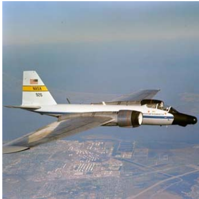
S73-36694.jpg - WB57-F Canberra, NASA 926; one of the planes used for remote sensing in the Earth Resources Program.
