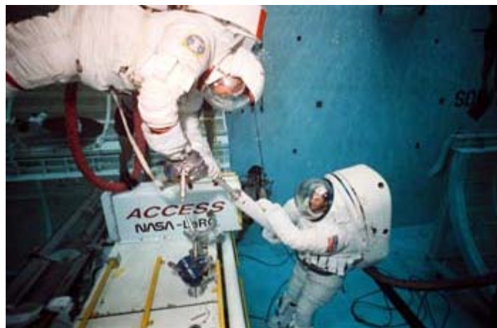
S89-38058.jpg - Underwater documentation using the AX-5 and MK III 8.3 PSI suits and the Space Shuttle 4 PSI suit in WETF evaluation runs, May 1989.
