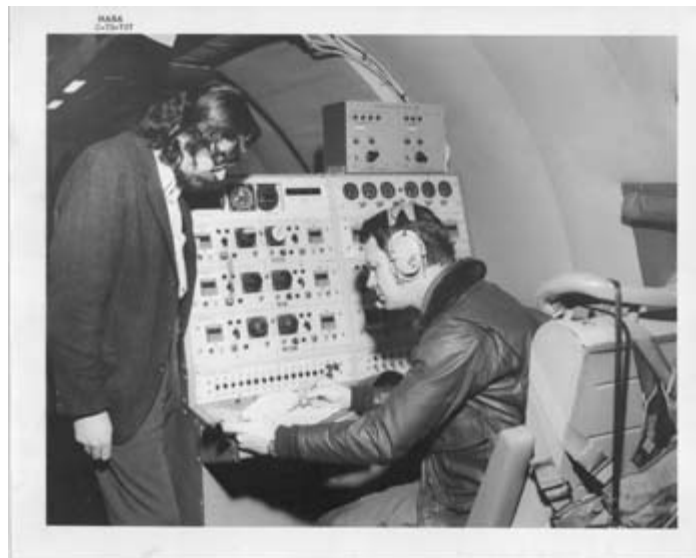
C-72-797.jpg - Console used to remotely control multispectral cameras, a bank of six cameras that shot infrared and regular film, both color and black-and-white, for the JSC Earth Resources Program.
